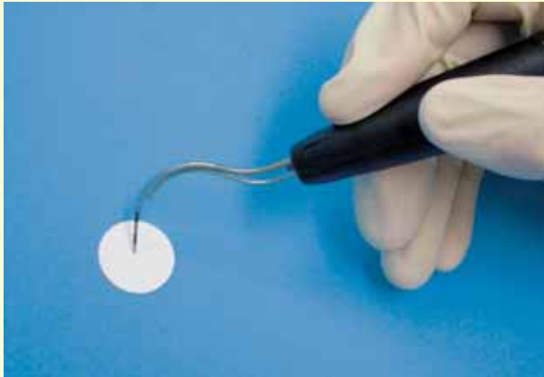
Fig. 5 System self-check: Tip of the probe placed on the testing standard. Single, brief tone: The system is ready for use. Multiple tones: The system is not ready for use.
