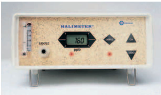
Fig 2 Halimeter® to determine the VSC in breath. With kind permission of Anysco Inc., Karlsruhe, Germany.
